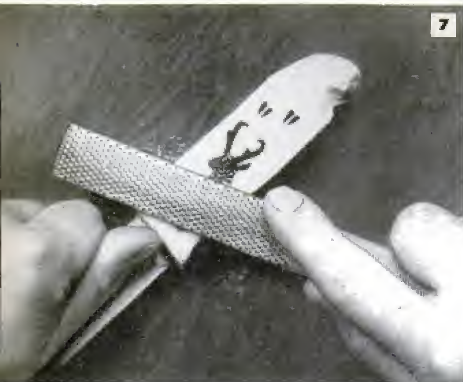
Plastic handle is a crude block when foil is removed from it. This is roughed to shape with wood rasp or coarse sandpaper
